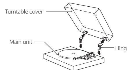
**1 Insert the hinges completely into the hinge holders at the left and right ends of the back of the main unit.**
